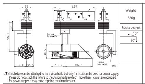
Input voltage 220V 50/60Hz Input current 0.071A Input wattage 15.1W
