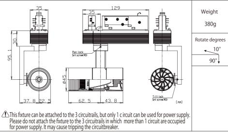
Input voltage 220V 50/60Hz
