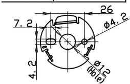
The hole for wire on the board  $\phi 13$
